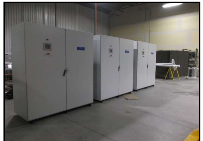
100 kW CW L-Band Microwave Transmitters, Designed and Built at Micronetixx for use in Microwave Plasma Energy Gas Processing, (Two Images Above)
