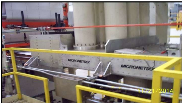
Image of the TM_{01} Mode Microwave 300 kW Heating Cell Ready for Start-Up for the Manufacture of Laminated Veneer Lumber, (LVL)
