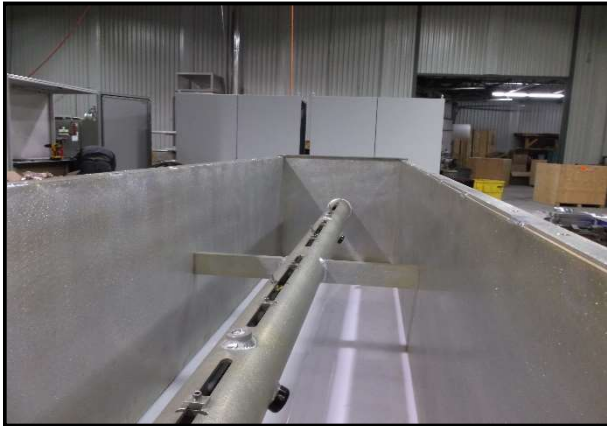
Close-up Image of a Medium-Power Special Extremely-Narrow Azimuth Beam UHF, (Channel 38), DTV Medium Power Transmitting Antenna
