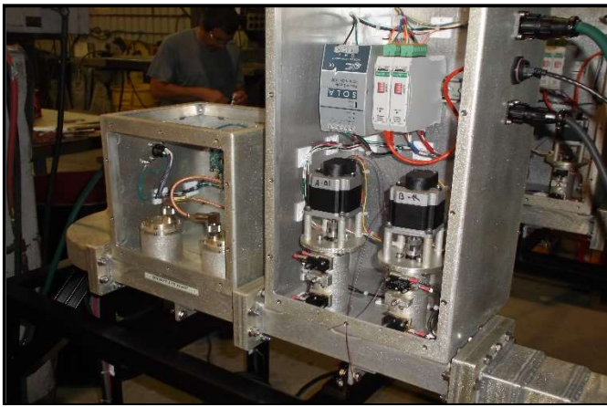
Integrated S-Band Waveguide AntiLog Sensor Instrumentation and Precision PLC-Controlled Zero-Backlash Stepper Motor-Actuated Auto-Tuning System
