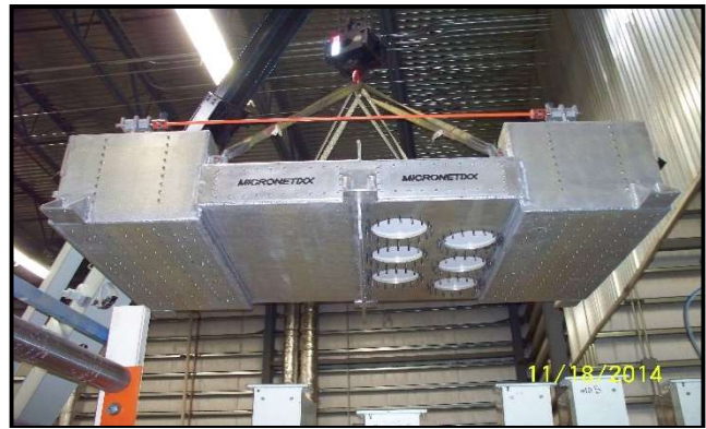
Micronetixx 300 kW CW TM_{01} Mode LVL Microwave Pre-Heating Cell Being Lowered Into Position on the Production Line
