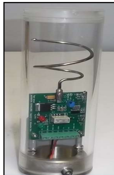
Micronetixx High-Power Microwave Power Density Safety Sensor/Monitor
