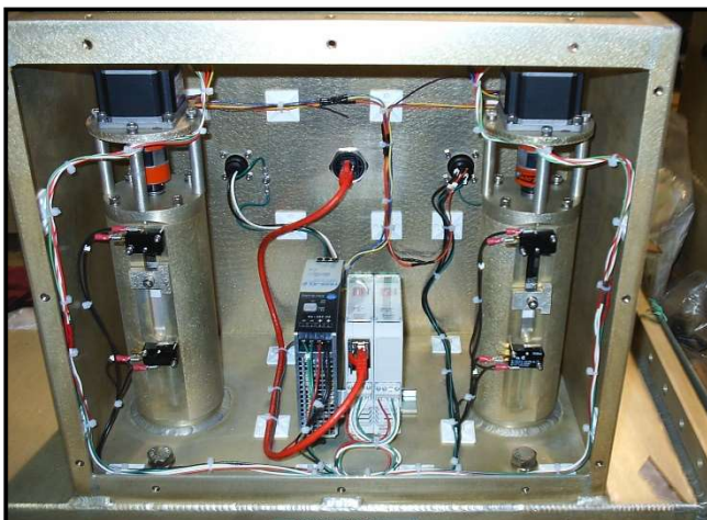
Micronetixx Precision Ethernet High-Power Waveguide 4-Axis Auto-Tuner With Stepper Motor Computer/PLC Dynamic Control
