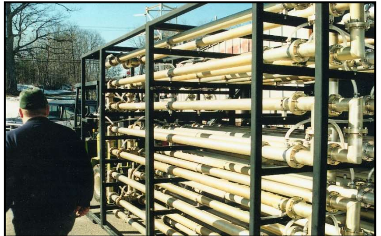
HF, High-Power Isolated 10:1 Bandwidth 60 kW Amplifier Combiner for White Sands
