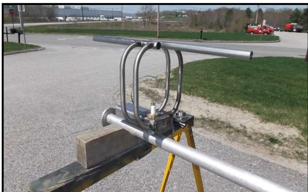
Micronetixx Model FMM Circularly-Polarized FM Radio Broadcast Antenna (Single-Element Characterization)
