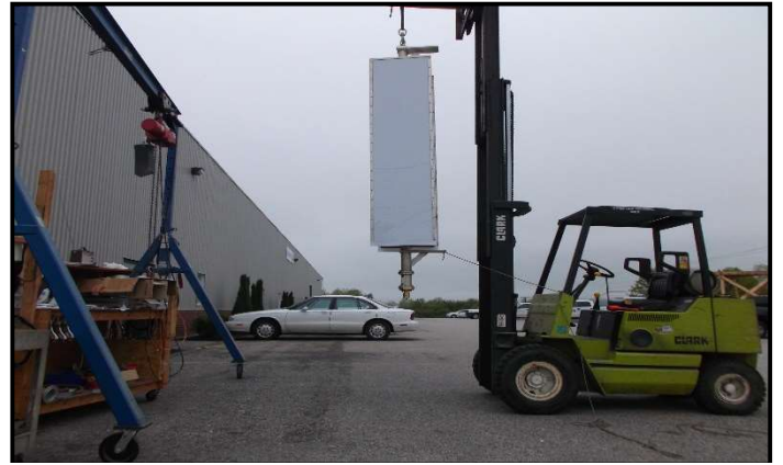
Special Medium-Power Channel 38 DTV Broadcast Antenna Being Moved to the Test Area for Final Testing
