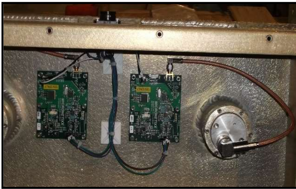
A Close-up of Micronetixx Anti-Log Power Microwave Sensing Modules Installed in a Precision Micronetixx Dual- Directional Coupler
