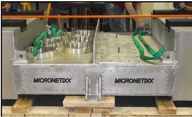
300 kW CW Industrial Microwave Pre-Heating System Being Readied for Installation at Pacific Woodtech Corporation in Burlington, Washington
