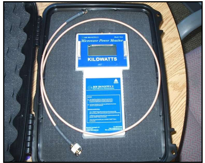
Micronetixx Model 714A/B Portable Microwave/RF Digital Power Meter With its Carrying Case
