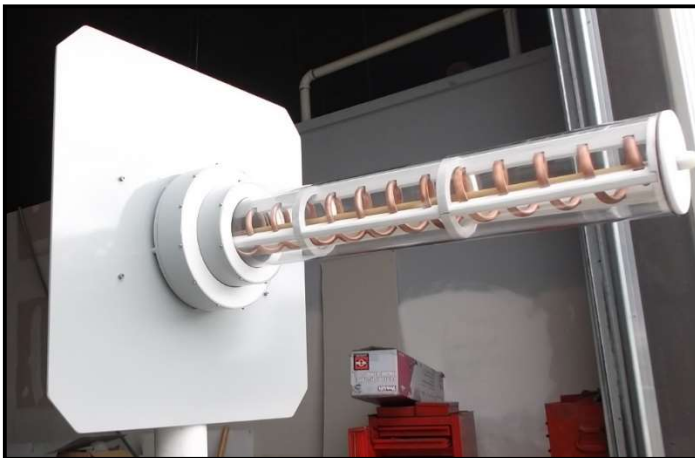
Special-Application High-Power/High Gain/High-Directivity Circularly-Polarized Antenna for the U.S. Military
