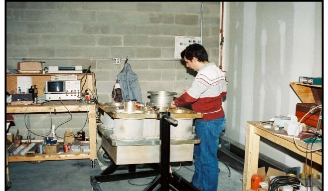
4-Port Motorized 50 Ohm High-Power (3 MW), Motorized Coaxial Transfer Switch for M.I.T.'s Plasma Fusion Center
