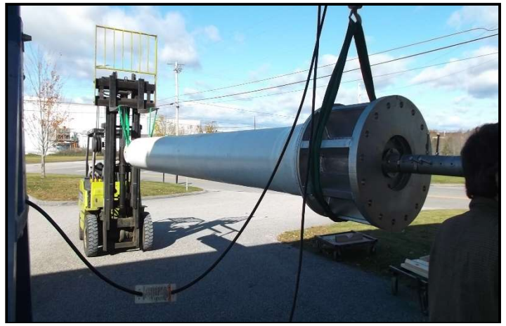
Completed High-Power SFN, (Reduced-RFR), DTV Antenna Being Transferred to the Test Area for Final Test and Plotting
