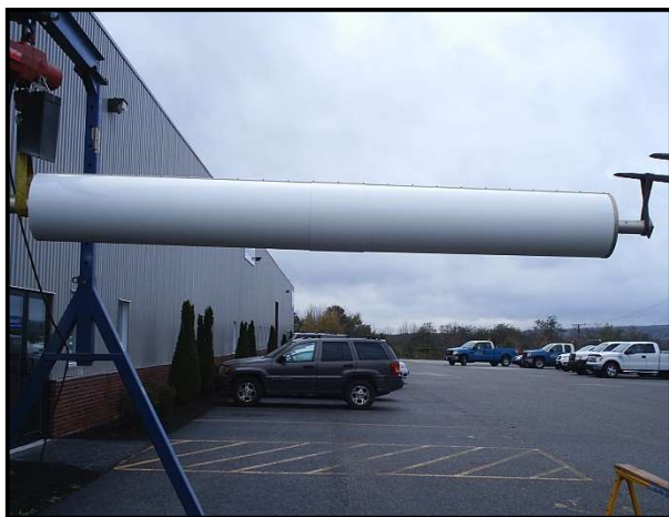
A DTV Medium-Power Broadcast Transmitting Antenna Being Moved to the Test Stand for Final Testing
