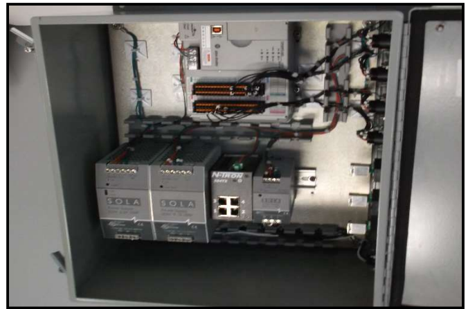
Micronetixx RF/Microwave AntiLog Sensing and Ethernet PLC Auto-Tuning Real-Time Monitor & Control System; Small Enclosure, (Interior)
