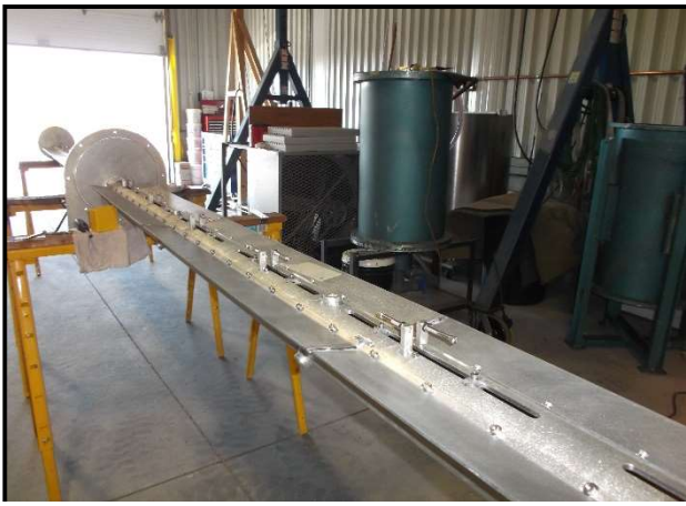
DTV Channel 50 Elliptically-Polarized, Pressurized-Radome Pylon before Radome Installation
