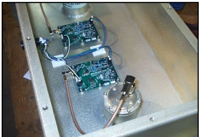
High-Power Waveguide Microwave Power Instrumentation, (Dual- Directional Couplers With Micronetixx Precision Anti-Log Sensing Modules)
