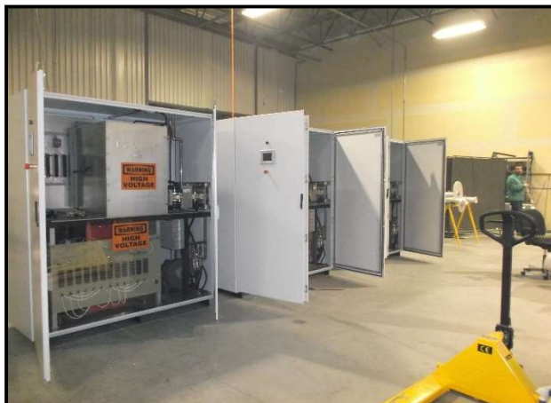
100 kW CW L-Band Microwave Transmitters, Designed and Built at Micronetixx for use in Microwave Plasma Energy Gas Processing, (Two Images Above)
